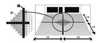
Implementation along a wall: start in the middle of the wall. Install the stair tiles on both sides
